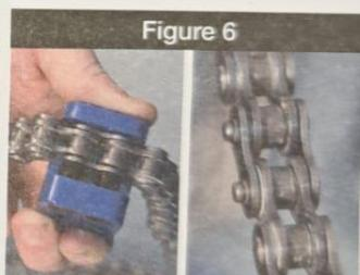
**Warning:** Do not overtighten! Overtightening the master link plate can damage the o-rings and cause the chain to bind and cause chain failure. Chain failure can result in great bodily injury or death.
